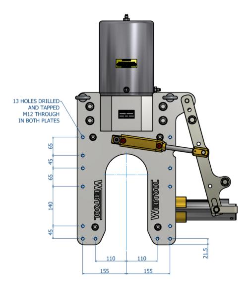
Two hydraulic supplies are required, ported as shown below. The maximum working pressures are shown in the table below and pressure limiting valves must be fitted into the supply to limit the pressures to these levels.
