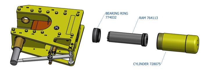
Figure 8 – Cylinder Removal
