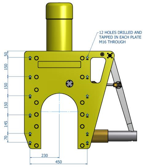
Figure 1 – Tool Mounting Holes
