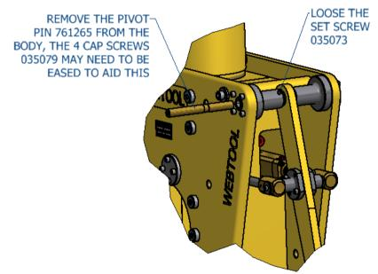
The lever will now be free, lift it free from the anvil SSC6489 The anvil SSC6489 may now be removed from the body. Re-assembly is the reverse of the above process.
