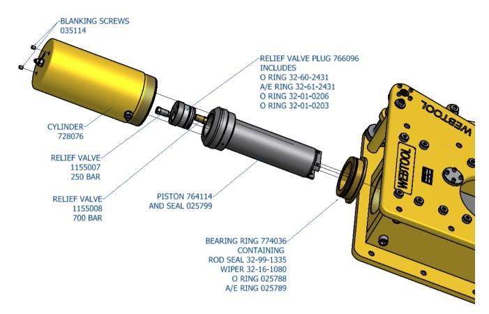
Removing the cylinder will expose the ram, bearing ring and relief valve plug and allow access to all the seals, note the positions of the relief valves and ensure they are replaced in the correct positions.
