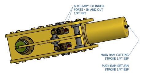
A relief valve should also be incorporated in the return line. This is to prevent excessively high pressures in the annular side of the hydraulic cylinders should the return to tank become blocked for any reason.
