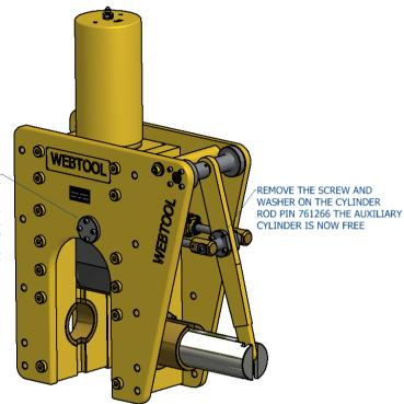
FREE THE LEVER AS DESCRIBED-IN SECTION 7 REMOVE 4 SCREWS 035079 AND MOUNTING STUD 079044 REMOVE THE SCREW AND WASHER ON THE CYLINDER ROD PIN 761266 THE AUXILIARY CYLINDERS ARE NOW FREE
