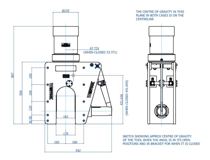
Above shows the centre of gravity of the tool for reference
