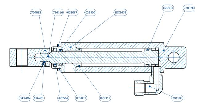
Above shows the part numbers for all the parts used in the auxiliary cylinders 982132 Page 12 of 16
