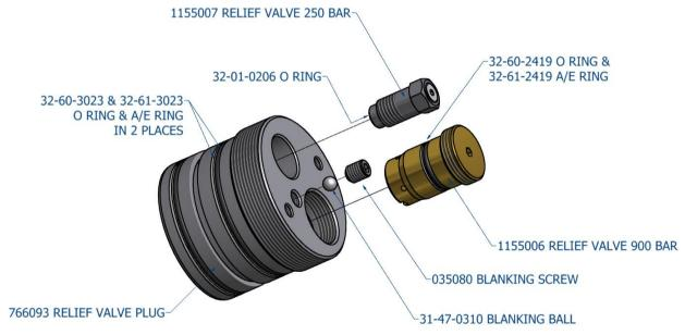
When re assembling the relief valve plug with the ram, first fill the ram with oil to the bottom of the counterbore, smear silver goop on to the threads of the plug, screw in the plug, remove the set screw and ball in the top of the plug and top up the inside of the ram with oil until it fills the screw hole, fit the ball and screw and lock tight.
