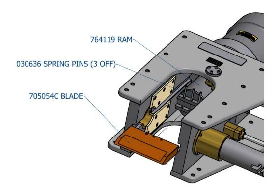
With the pins removed the blade can be taken from the cutter, gloves should be worn to prevent cuts from any sharp edges that may be present on the blade after use.
