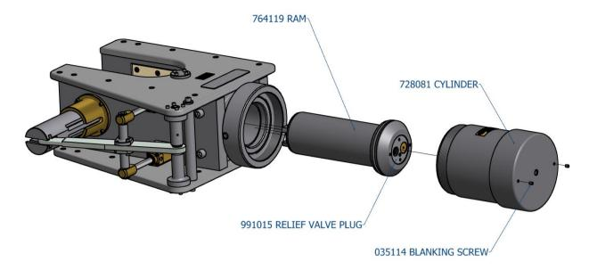
Put the assembled parts into a plastic dust bin or similar vessel, fit the coupling to the top of the cylinder, attach a hand pump to the coupling and pump out the ram, importantly, **by hand.** The ram will now be free of the cylinder and all seals will be accessible.
