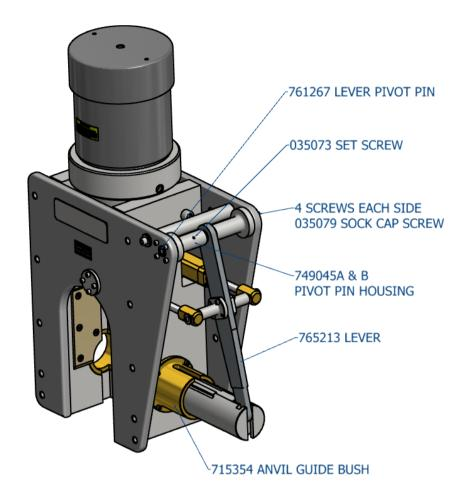
Withdraw the pivot pin 761267 far enough to release the lever arm. (There is an M6 tapped hole in the end of the pivot pin to assist in withdrawing this)
