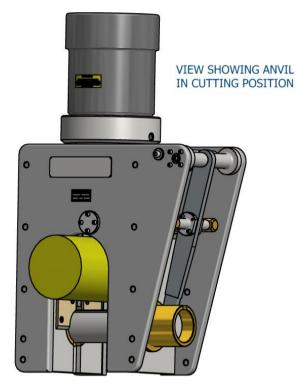
Operate the main ram down-stroke to sever the wire rope. Once the wire rope is severed, Pressurize the main ram retract port to withdraw the cutting blade. Then, and only then, retract the anvil. It is important not to operate the anvil cylinder whilst the main ram and blade are in the fully extended position.
