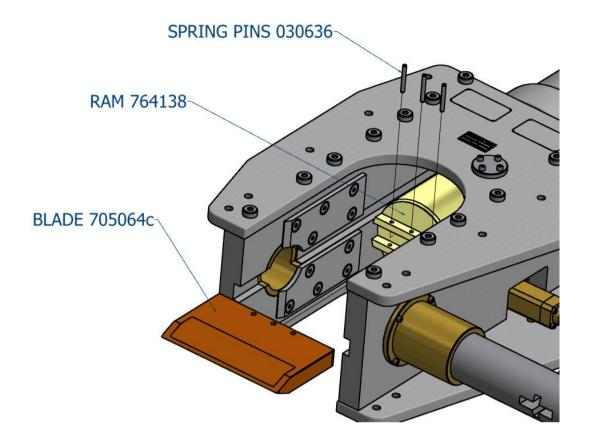
With the pins removed the blade can be taken from the cutter, gloves should be worn to prevent cuts from any sharp edges that may be present on the blade after use.
