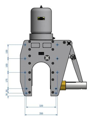
Two hydraulic supplies are required, ported as shown below. The maximum working pressures are shown in the table below and pressure limiting valves must be fitted into the supply to limit the pressures to these levels.
