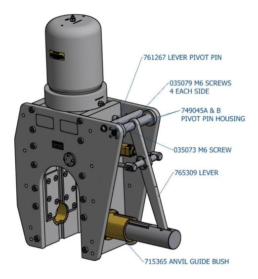
Withdraw the pivot pin 761267 far enough to release the lever arm. (There is an M6 tapped hole in the end of the pivot pin to assist in withdrawing this)
