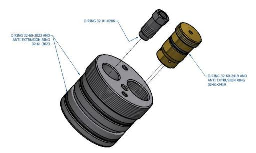
When re assembling the relief valve plug with the ram, first fill the ram with oil to the bottom of the counterbore, smear silver goop on to the threads of the plug, screw in the plug, remove the set screw and ball in the top of the plug and top up the inside of the ram with oil until it fills the screw hole, fit the ball and screw and lock tight.
