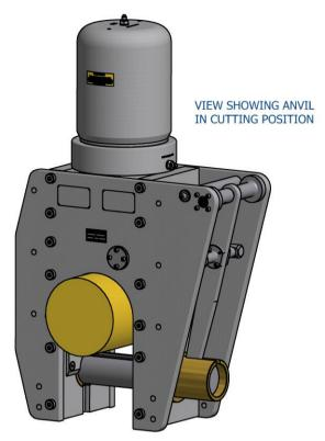
Operate the main ram down-stroke to sever the wire rope. Once the wire rope is severed, Pressurize the main ram retract port to withdraw the cutting blade. Then, and only then, retract the anvil. It is important not to operate the anvil cylinder whilst the main ram and blade are in the fully extended position.
