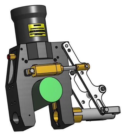
Pressurize the auxiliary cylinders to fully extend the anvil, thus retaining the material in the body of the tool. Check visually that the anvil is fully home, this is important to prevent damage to the tool.
