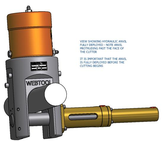
Operate the main ram power port to sever the wire rope, hold pressure until the wire rope is severed.
