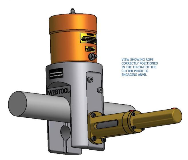
Pressurize the anvil cylinder to fully extend the anvil, thus retaining the wire rope in the body of the tool. Check visually that the anvil is fully home, this is important to prevent damage to the tool (The end of the anvil should just be proud of the body of the tool on the opposite face to the anvil cylinder).
