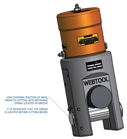
Operate the main ram power port to sever the wire rope, hold pressure until the wire rope is severed.
