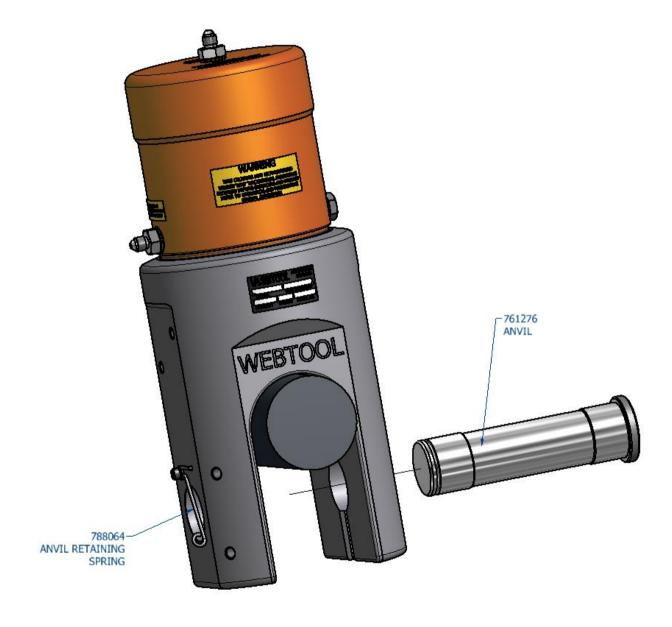
Replace the anvil 761276 and ensure the anvil retaining spring 788064 is located thus retaining the wire rope in the body of the tool. It is important that the anvil is correctly located i.e. the spring is located in the groove in the anvil, this will prevent damage to the tool.
