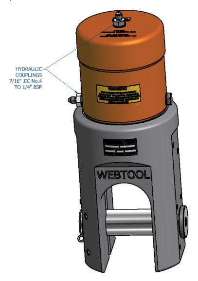
A relief valve should also be incorporated in the return line. This is to prevent excessively high pressures in the annular side of the hydraulic cylinders should the return to tank become blocked for any reason.
