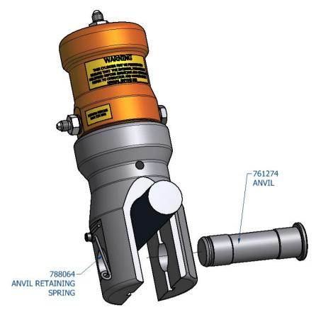
Replace the anvil 761274 and ensure the anvil retaining spring 788064 is located thus retaining the wire rope in the body of the tool. It is important that the anvil is correctly located i.e. the spring is located in the groove in the anvil, this will prevent damage to the tool.
