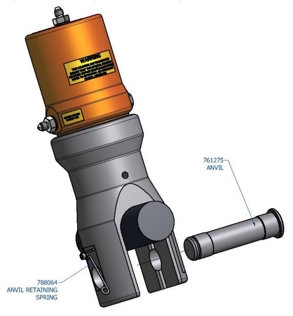
Replace the anvil 761275 and ensure the anvil retaining spring 788064 is located thus retaining the wire rope in the body of the tool. It is important that the anvil is correctly located i.e. the spring is located in the groove in the anvil, this will prevent damage to the tool.
