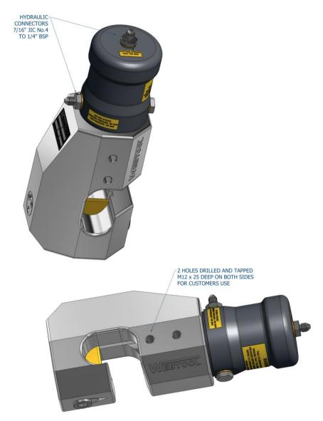
A hydraulic supply is required, ported as shown. The maximum working pressures are shown in the table 1 below and pressure limiting valves must be fitted into the supply to limit the pressures to these levels.
