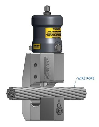
Place the wire rope in the cutter. Ensure that the wire rope is as far into the cutter as possible.
